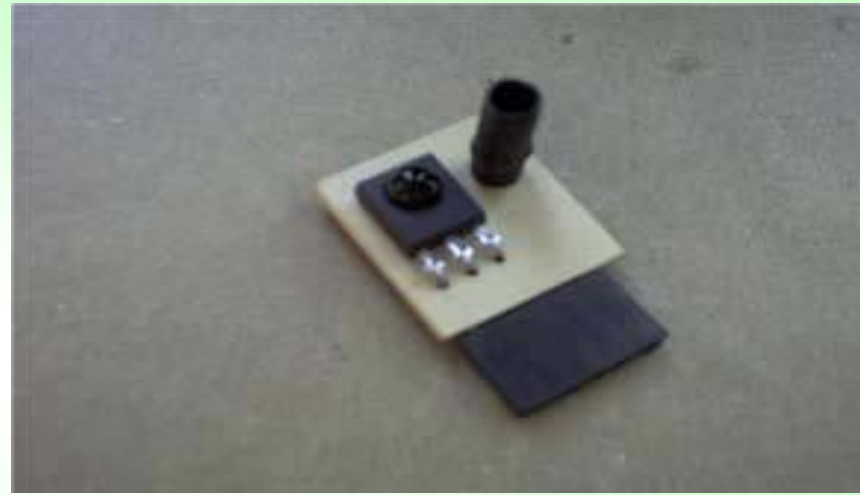
Fig. 12: IR receiving and transmitting diode
