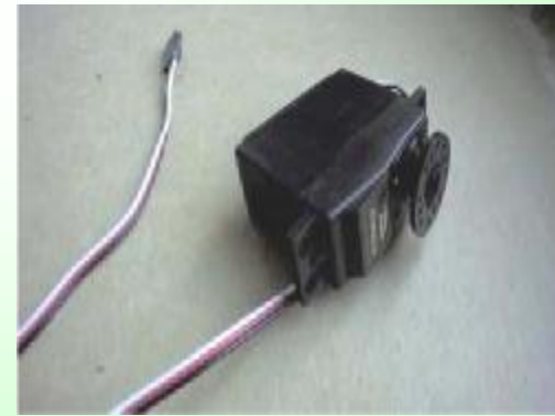
Fig. 10: Servo motor of R/C models and an element that can be used as a wheel
