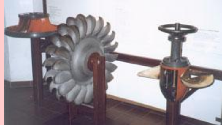
Photo 10: Runner of Pelton turbine
